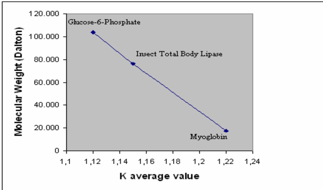
**Figure 2:** Graphic of K average ( $K_{av}$ ) values-molecular weights of Myoglobin, Glucose-6-phosphate and purified insect total body lipase.
