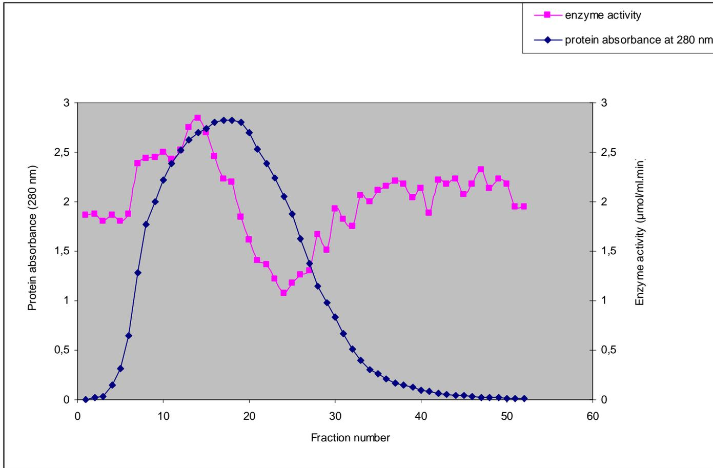
**Figure 1:** Sephadex G-100 column gel filtration chromatography elution profile
